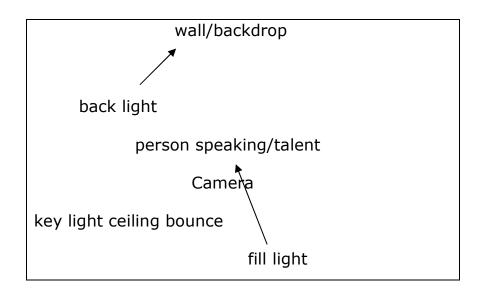
Take your key light and put it directly in front of the person talking and shine it up to a ceiling (presuming you are inside) so it hits your white ceiling and bounces down. This causes a nice blend without hard shadows. It doesn't really matter if your ceiling is shiny or not, the point is to spread more even light that matches the color temperature you are using for the other lights.
