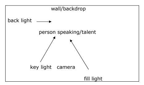
Put the key light to the left of the camera and raise the light 45 degrees from the talents' head.
